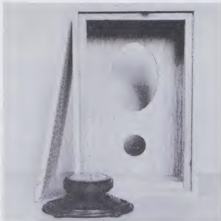
Fig. 15-24. Project 8: Enclosure minus duct and damping material. Speaker is front mounted.
