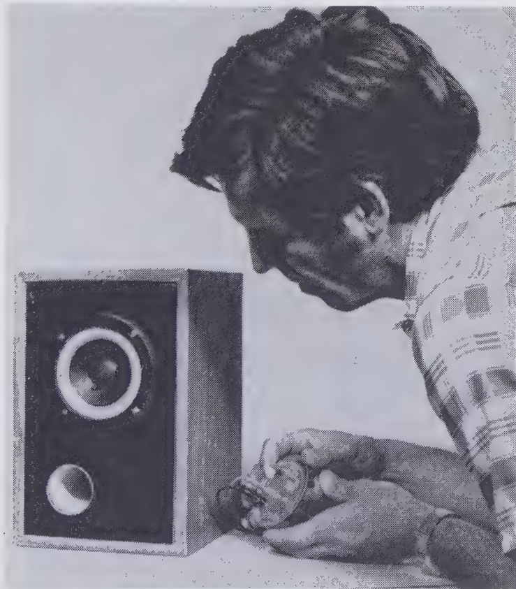
Fig. 3-20. Tests 13 and 19 can be made with a simple polarity/damper tester diagrammed in Test Set-up F. (Project 15 being tested.)
