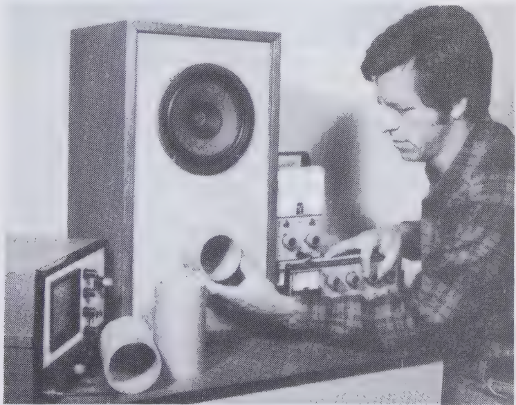
Fig. 7-7. The easiest way to tune a ported box is with the duct outside the box so you will not have to remove the back every time you change the duct length.
