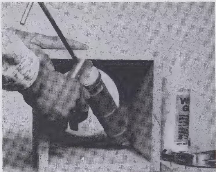
Fig. 3-3. Making a standard test box. Caulk all the interior joints before gluing and nailing on the bottom, then caulk the bottom through speaker hole.
