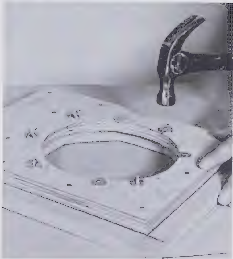
Fig. 4-12. Driving T-nuts into back of speaker board to receive 3 16 in. machine screws (Project 10).
