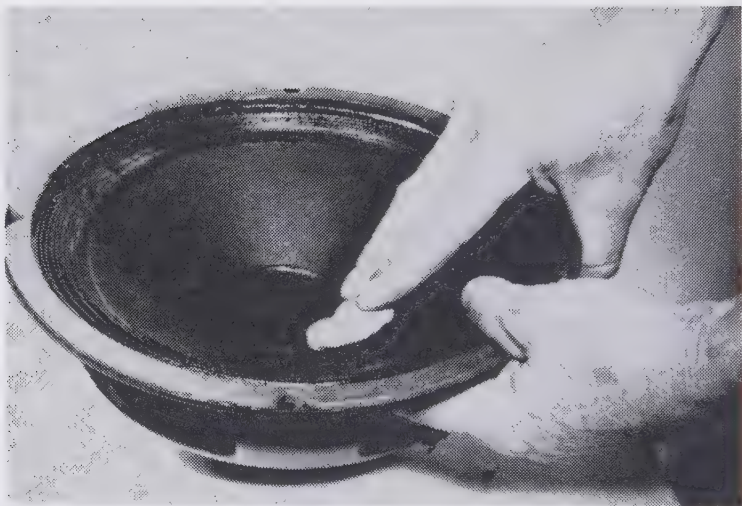
Fig. 3-10. Support the woofer cone with one hand while you press down a blob of modeling clay with the other.
