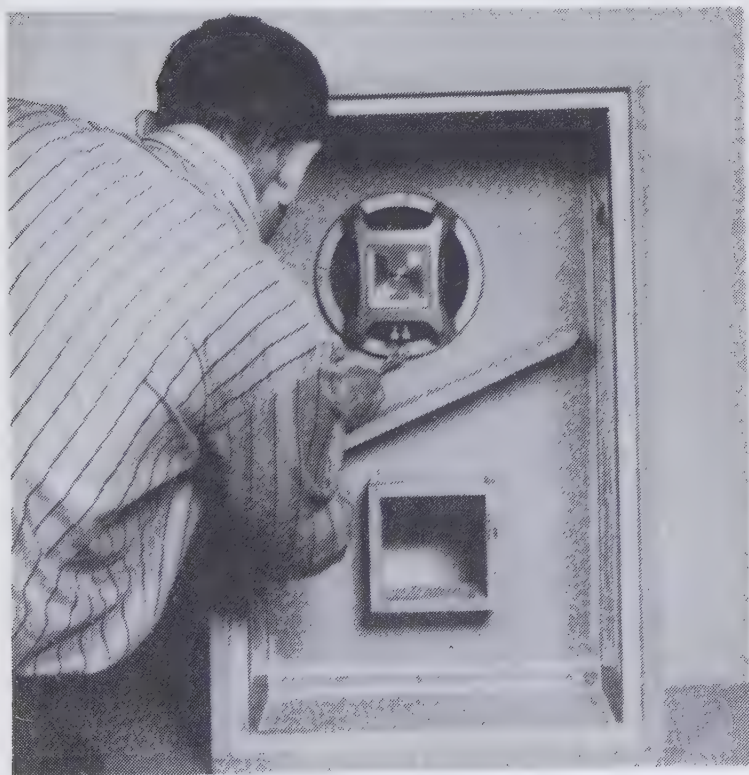
Fig. 15-18. Project 6: Installing Electro-Voice speaker. Tighten nuts snugly to compress gasket, but do not use heavy force, or you might bend frame.
