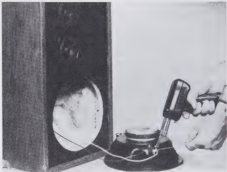
Fig. 15-13. Project 4: The final step is wiring and installing the woofer. Note color coded wire to make phasing easy.
