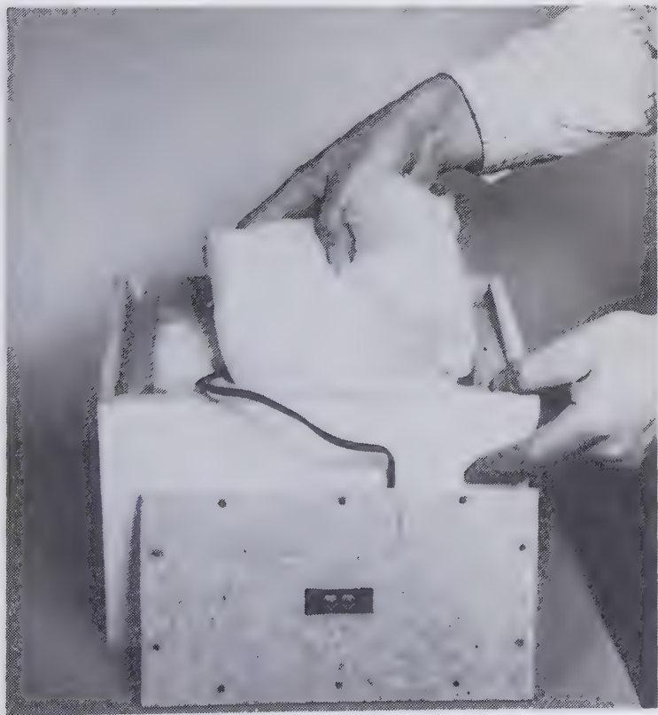
Fig. 4-14. Most miniature closed boxes should be filled with damping material. Note terminal strip on back (Project 17).
