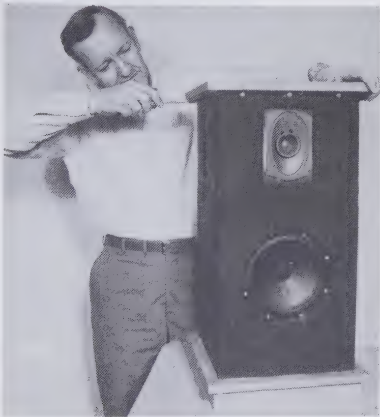
Fig. 9-4. Project 10. Screws through the sides hold down the top. The super tweeter is in the rear.
