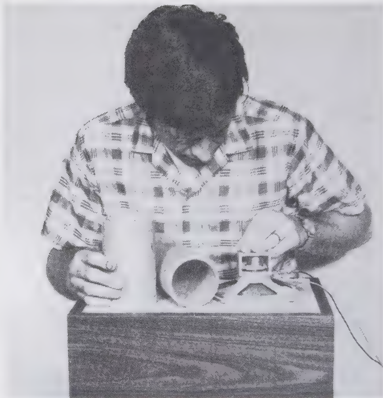
Fig. 7-8. Tuning a ported box by Test 7, Method IV: the listening method, using a cheap speaker.
